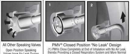
Valves have Air Leak During Exhalation and Do Not Provide a Closed Respiratory System.
